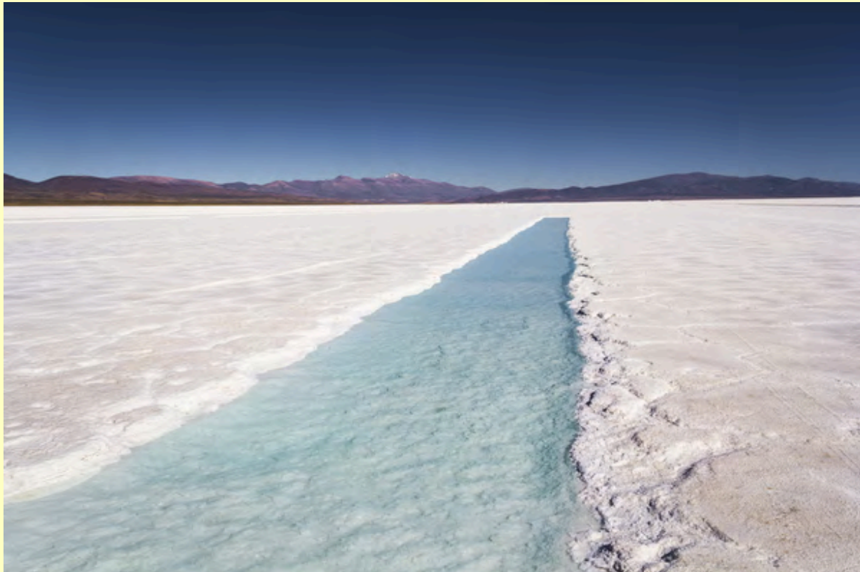
BrinBrine is extracted from salt water flats in South America to obtain lithium. (Credit: Klaus Balzano/Shutterstock)
